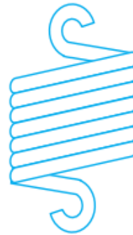
(b) tension helical spring
